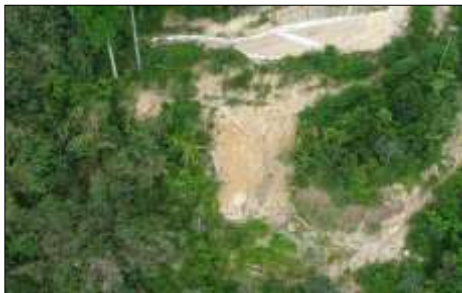
Temporary Soil Stabilization Not Done in Exposed Areas Transmission Line Project Causes Soil Erosion and Landslides
